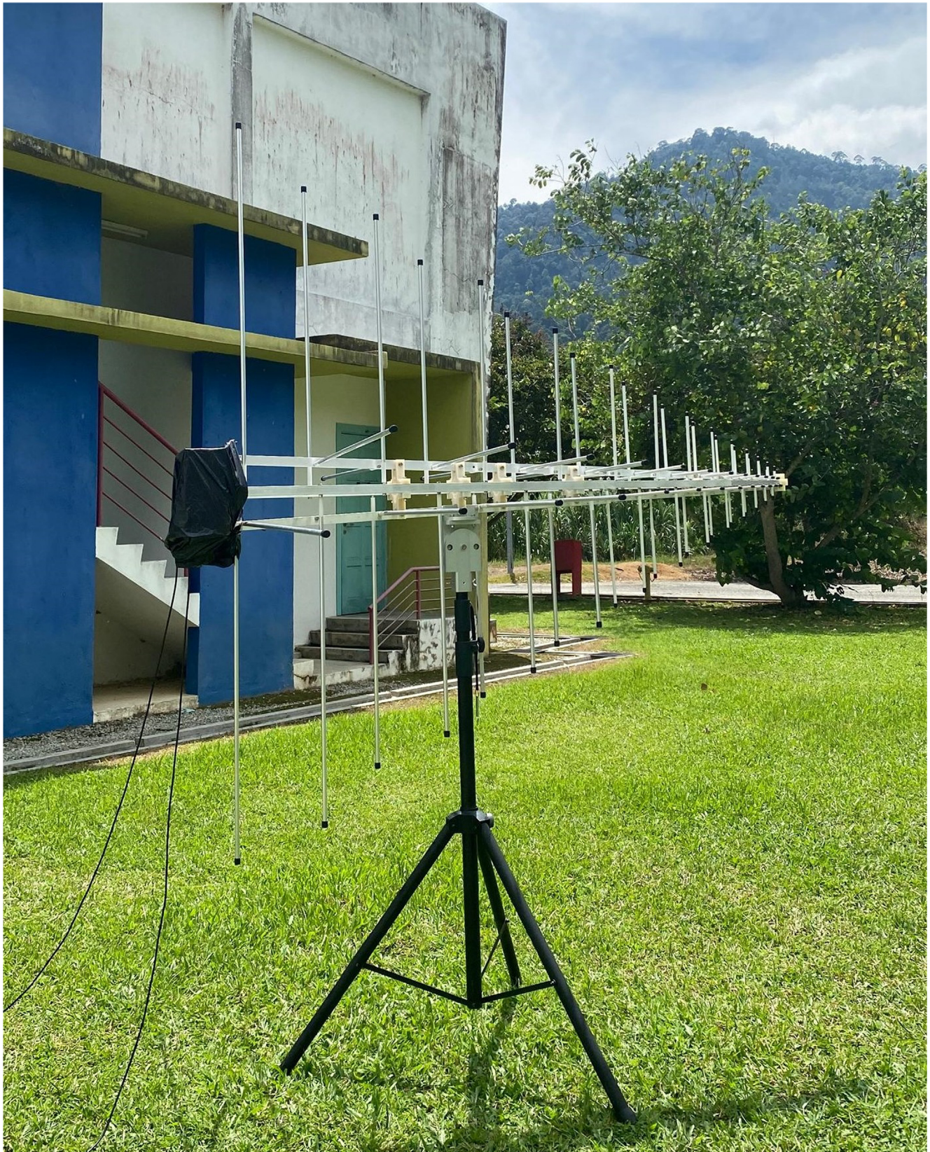
Fig. 3. Side-view of the dual-polarization logarithmic periodic antenna set up in GL for radio observation. The two coaxial cables connected to the base of the antenna are connected to the spectrum analyser.
